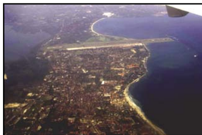
Fig. 7. International Airport Bali: the runway has been extended by several hundred meters to the west, in order to provide for large aircraft like the 747. A beautiful reef, right in the tourist centre Kuta, has been sacrificed.
